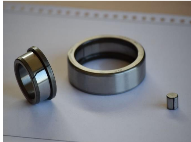
Figure 2. Defective Bearing Components.
