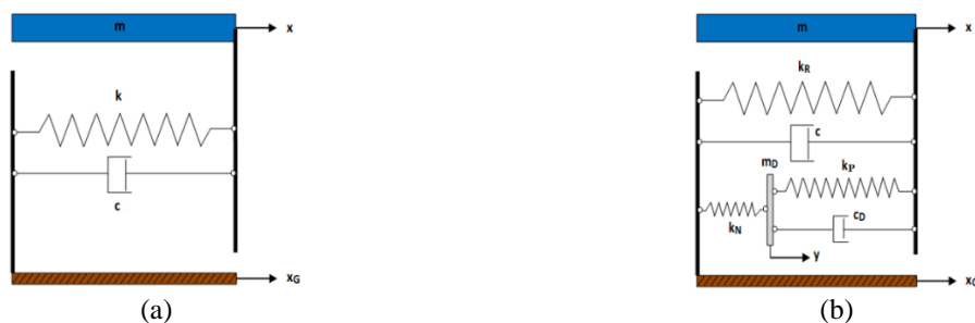
Figure A.1. (a) Undamped (or low damped) SDOF system and (b) schematic representation of the KDamper concept.
