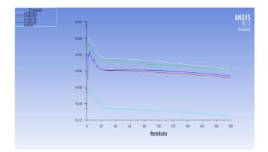
Figure 14. Residual iterations for ANSYS FLUENT simulation (TiO<sub>2</sub> nanofluid,  $\Phi = 0.1$ ).
