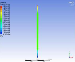
Figure 11d. Pressure Contours for TiO<sub>2</sub> nanofluid,  $\Phi = 0.01$ .
