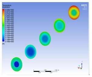
Figure 8b. Temperature Contour cross sections for  $Al_2O_3 \ nanofluid, \ \Phi=0.01. \label{eq:alpha}$
