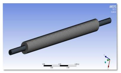
Figure 2. ANSYS FLUENT 3-dimensional mesh of solar configuration (Mesh density Nodes: 479188, elements: 443970).
