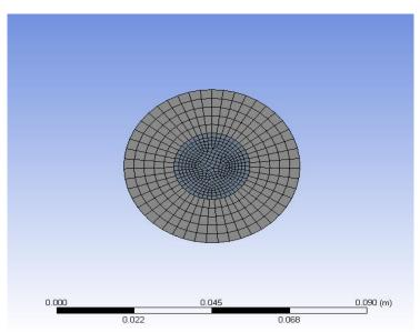
Figure 3. ANSYS FLUENT cross-sectional meshing details.
