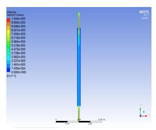
Figure 10c. Velocity Contours for Al<sub>2</sub>O<sub>3</sub> nanofluid,  $\Phi = 0.1$ .
