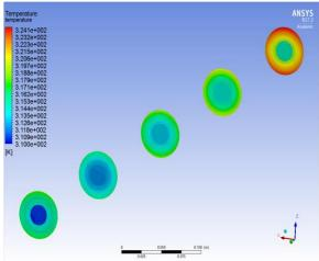
Figure 9b. Temperature Contour cross sections for  $Al_2O_3 \ nanofluid, \ \Phi=0.05.$
