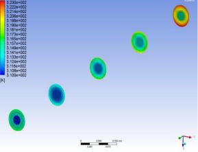
Figure 11b. Temperature Contour cross sections for  $TiO_2 \text{ nanofluid}, \Phi = 0.01.$
