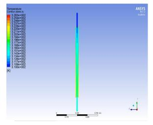
Figure 13a. Temperature Contours for  $TiO_2$ nanofluid,  $\Phi = 0.1$ .
