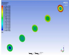
Figure 7b. Temperature Contour cross sections for CuO nanofluid,  $\Phi = 0.1$ .
