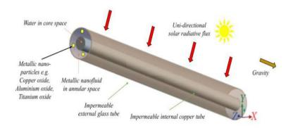
Figure 1. Geometrical and physical model for annular nanofluid solar collector.
