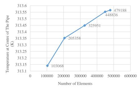
Figure 4. ANSYS FLUENT grid independence study.
