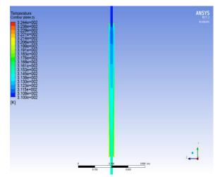
Figure 9a. Temperature Contours for  $Al_2O_3$ nanofluid,  $\Phi = 0.05$ .
