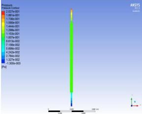
Figure 13d. Pressure Contours for TiO<sub>2</sub> nanofluid,  $\Phi = 0.1$ .
