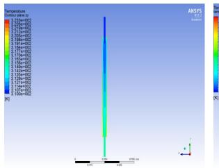
Figure 11a. Temperature Contours for  $TiO_2$ nanofluid,  $\Phi = 0.01$ .
