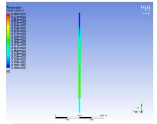
Figure 7a. Temperature Contour for CuO nanofluid,  $\Phi = 0.1$ .
