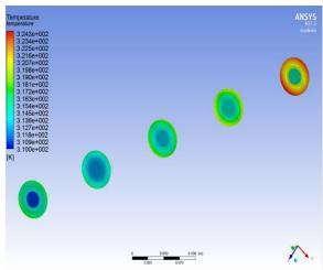
Figure 12b. Temperature Contours cross sections for  $TiO_2 \text{ nanofluid}, \ \Phi=0.05.$
