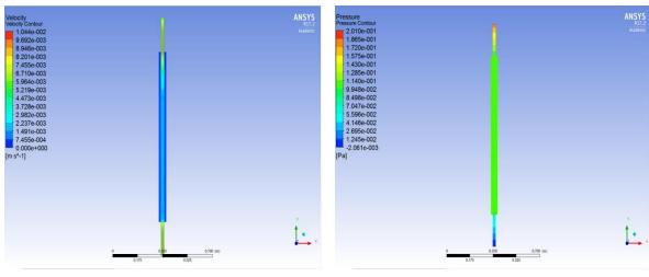
Figure 7c. Velocity Contours for CuO nanofluid,  $\Phi = 0.1$ .
