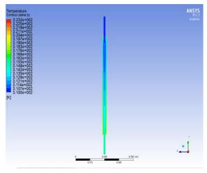
Figure 8a. Temperature Contour for  $Al_2O_3$  nanofluid,  $\Phi=0.01. \label{eq:phi}$
