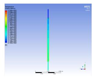
Figure 12a. Temperature Contours for  $TiO_2$ nanofluid,  $\Phi = 0.05$ .
